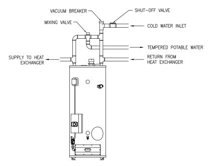
Suggested Piping Arrangement For Top Connections
